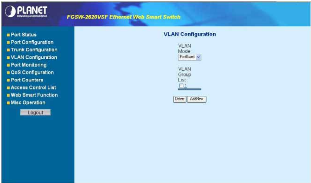
Figure 4-16 Port-based VLAN Setting Web Page screen
